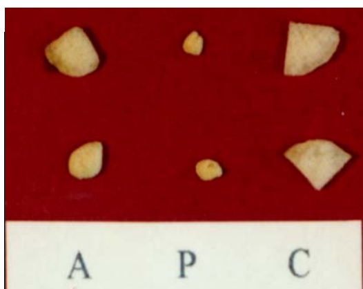
Figure 10. Acetic Acid (A), Propionic Acid (P), and Acetic Acid Control Scaffolds (C) After 4 Days
